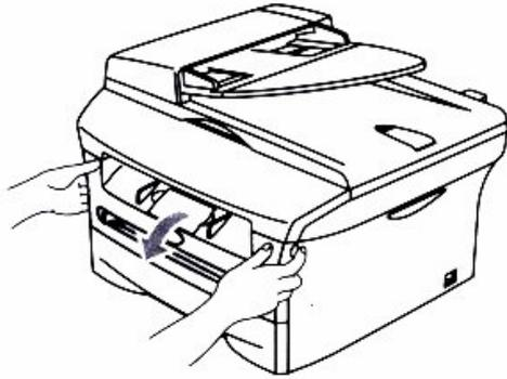
2. Pull out the drum unit and toner cartridge assembly.
