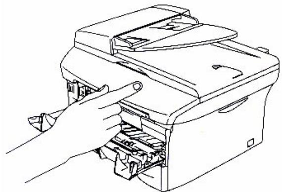
8. On MFC series printer, when "Replace Drum?" appears on the LCD, press 1. When "Accepted" appears, close the front cover.
