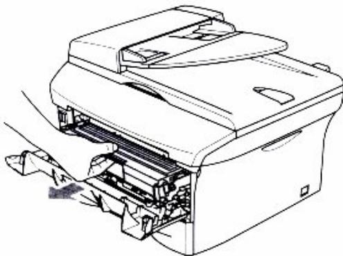
3. Push down the blue lock lever and take the toner cartridge out of the drum unit.
