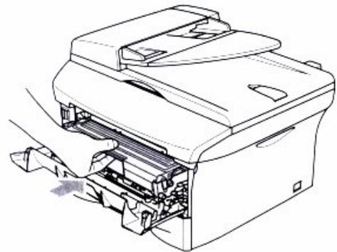
7. To reset the drum counter, make sure that the front cover is open and then press Options on the control panel.
