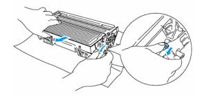
3. Push down the blue lock lever and take the toner cartridge out of the drum unit.
