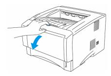
1. Open the front cover of the machine and pull out the drum unit assembly as shown in the picture.
