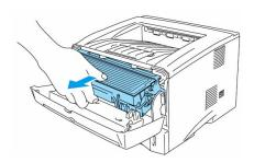
2. Pull out the drum unit assembly.
