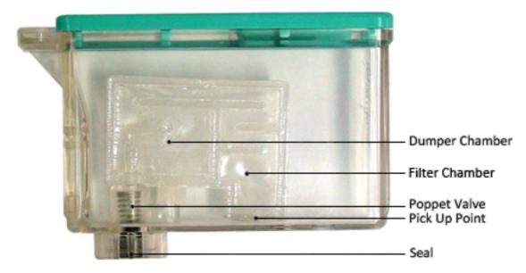
**How it works** - When the printer requires ink, it is pulled into the *filter chamber*, from the *pick up point*, then through the *damper chambers* and down past the *poppet valve* and into the printer.
