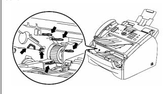
2. Hold down the lock lever on the left and pull the toner cartridge out of the drum unit.
