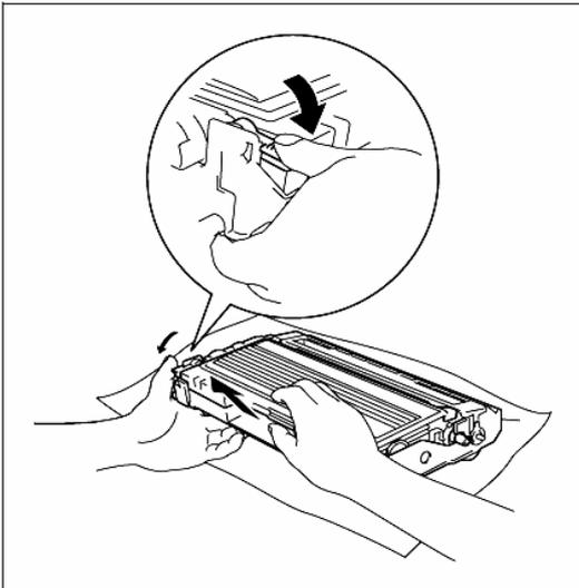
3. Push down the blue lock lever and take the used toner cartridge out of drum unit.
