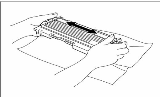
4. Unpack the new toner cartridge. Hold the cartridge level with both hands and gently rock it from side to side five or six times to spread toner evenly inside the cartridge.
