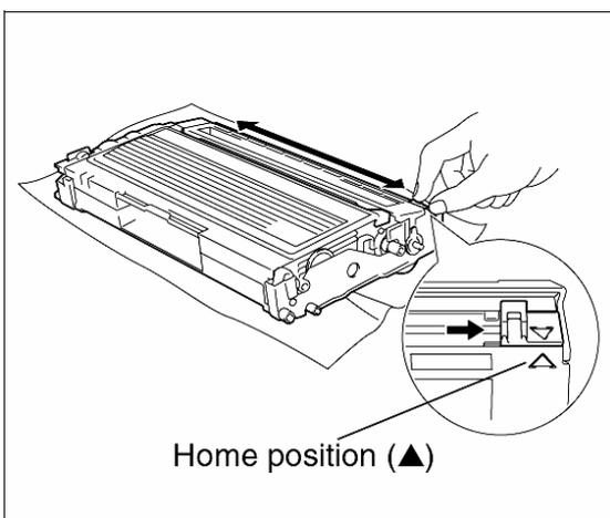
7. Clean primary corona wire inside the drum unit by gently sliding the blue tab from right to left and from left to right several times. Return the tab to the home position (▲) before you put the drum unit back to the printer. If you do not, printed pages may have a vertical stripe.
