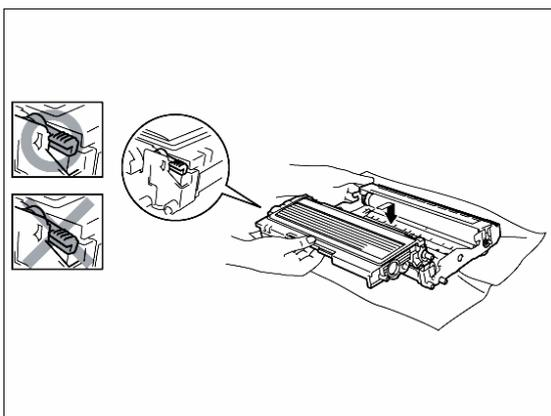
6. Put the new toner cartridge firmly into the drum unit until you hear it lock into place. If you put in properly, the lock lever will lift automatically.
