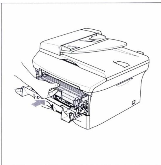
8. Put the drum unit and toner cartridge assembly back into the printer. Close the front cover of the printer.
