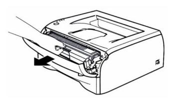
2. Push down the blue lock lever and take the toner cartridge out of the drum unit.
