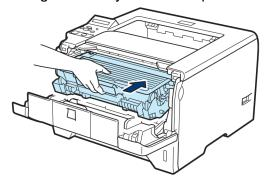
Hold down Go until the message DRUM CLEAR is displayed on the LCD, then release Go.
