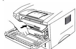
4. Re-install the drum unit assembly into the machine.
