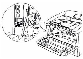
5. Keep holding down the button until all LEDs turn on with the front cover open, then release the button.
