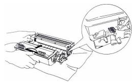
3. Unpack a new drum unit. Install the toner cartridge into the new drum unit it locks into place, indicated by a click.
