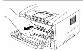
1. Open the front cover of the machine and pull out the drum unit assembly as shown in the picture.
