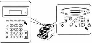
7. With front cover open, press the clear button on the control panel. Then, "REPLACE DRUM?" message appears on the LCD.
